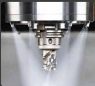
Air through nozzles
