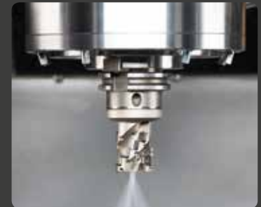
Air through spindle
